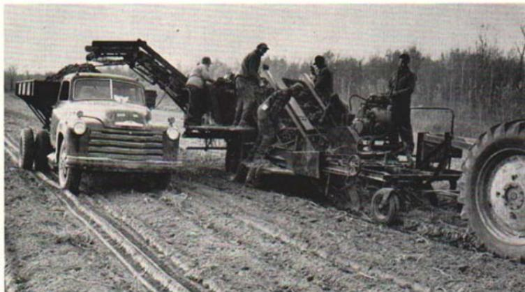
Fig. 9. A mechanical harvester in operation. A fairly small crew operate the machine that does the job of digging and loading into a self unloading box on the truck.
