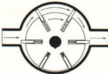
Fig. 11. — Sliding vane impeller pump.
