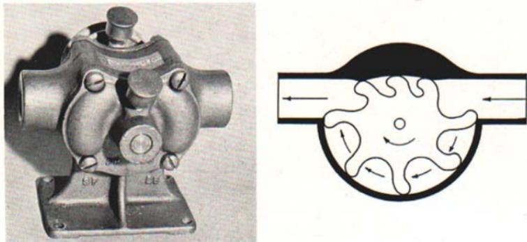
Fig. 9. — Flexible impeller pump.
