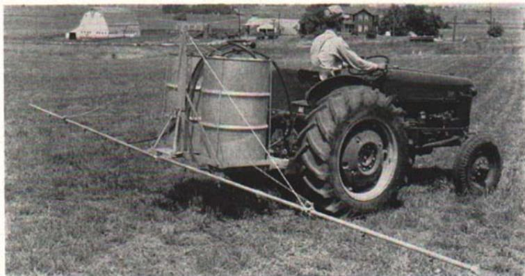
Fig. 4. — Tractor-mounted weed sprayer.
