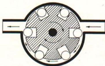
Fig. 10. — Roller impeller pump.
