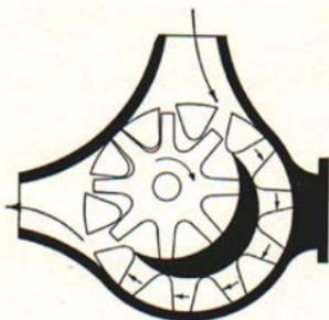
Fig. 13. — Internal idle gear pump.
