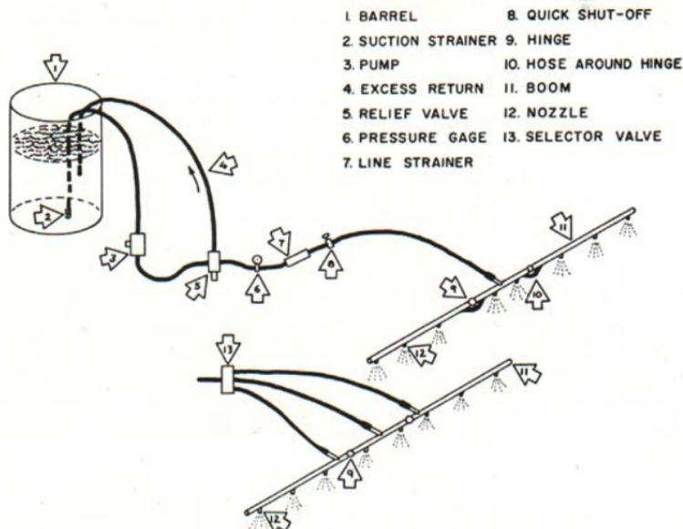
Fig. 6. — Layout of a boom weed sprayer.
