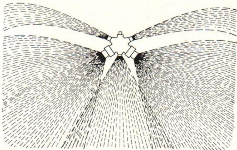
Fig. 19. — Spray pattern from a nozzle cluster.
