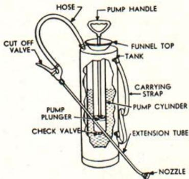
Fig. 1. — Compressed air hand sprayer.
