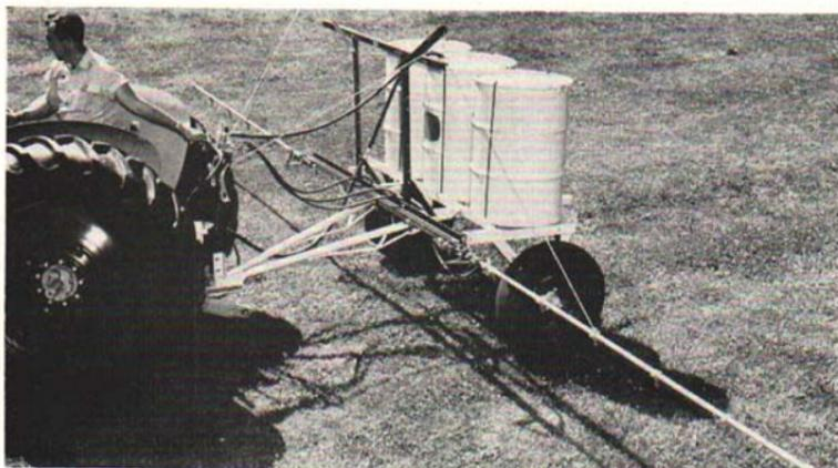
Fig. 5. — Trailing type weed sprayer with PTO pump.
