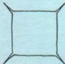
Fig. 1 Slashing corners for set-in patch.
