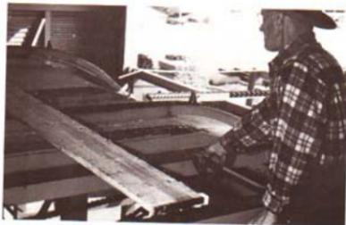
Fig. 22. Following the secondary manufacturing operations of surfacing and/or resawing, the lumber is sorted according to width, thickness, grade, etc. This view shows the sorter operator controlling the diversion of boards into a multideck sorter. The position of the slider bar operated by his right hand determines which level the board will seek. Each level of the sorter contains a particular grade or size of board. (Photo: The Ivory Pine Co.)
