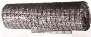
Fig. 34. This photograph illustrates the briquet made by the process shown in Figs. 27 and 31. The log produced measures 3¾ inches in diameter by 12 inches long and it weighs a little over 5 pounds. The ring structure of this log shows clearly in the photograph and is due to the manner in which the log is extruded through the single log tube. (Photo: Sumner Iron Works, a division of The Black Clawson Company).
