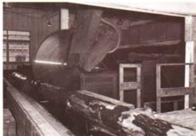
Fig. 9. Circular, 48-inch diameter swing cutoff saw with air feed cylinder. Log dogging jaws which will accommodate themselves to burly or uneven logs are visible to the left of the saw line. Here logs are bucked into exact lengths ranging from 8 to 12 feet to produce a multiple of the desired pallet board length. This equipment is located at D in Fig. 10. (Photo Sumner Iron Works, a division of The Black Clawson Company).
