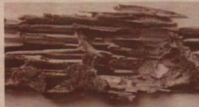
Termite damage. Note the "shelving" of the wood. Especially on the lower part of the picture, observe the corky material. This is yellowish and often black-specked. Carpenter ants "shelve" wood by feeding similar to termites, but a sawdust is present with carpenter ants, absent with termites. The sawdust of carpenter ants is coarse and often held together by a webbing secreted by the insects.
