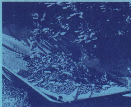
Figures 17 & 18 — (Left) Mechanical harvesting removes leaves and debris which must be separated from fruit after harvest. (Right) Mechanical fingers vibrate berries from canes onto collecting pans and conveyors beneath the bush.
