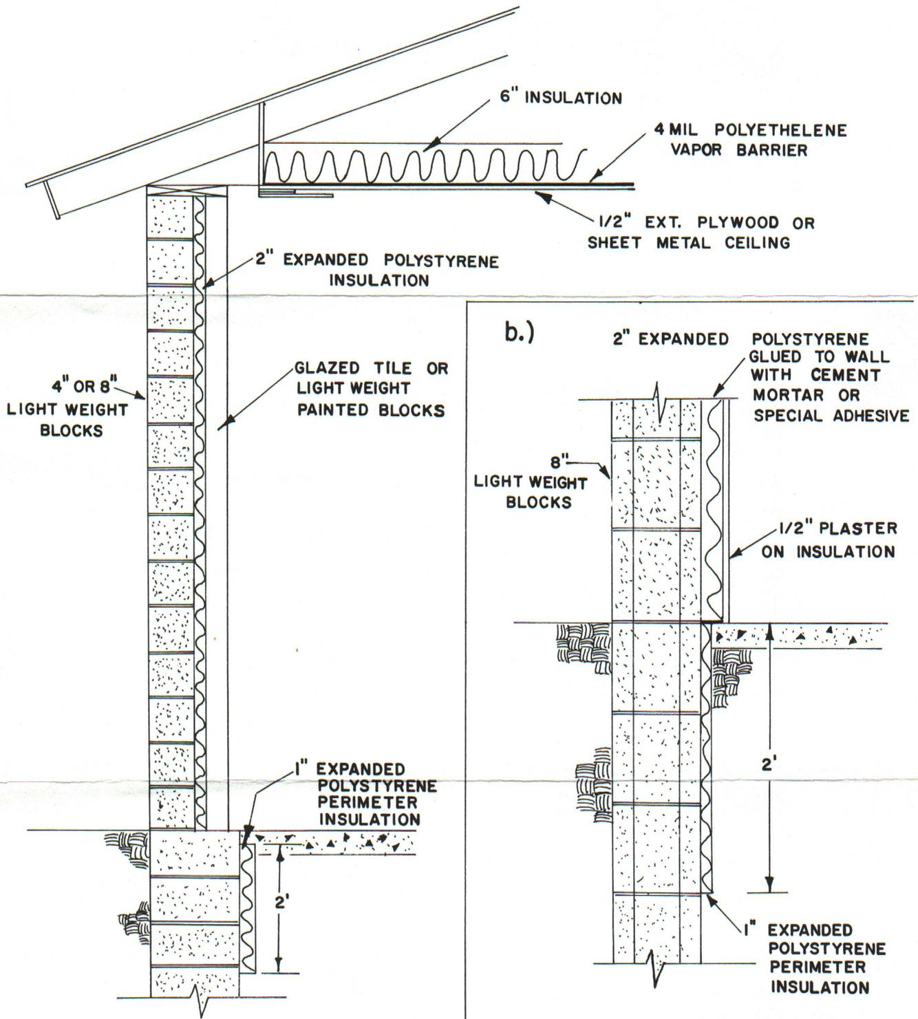
Fig. 2 CROSS-SECTION OF MASONRY WALL CONSTRUCTION
