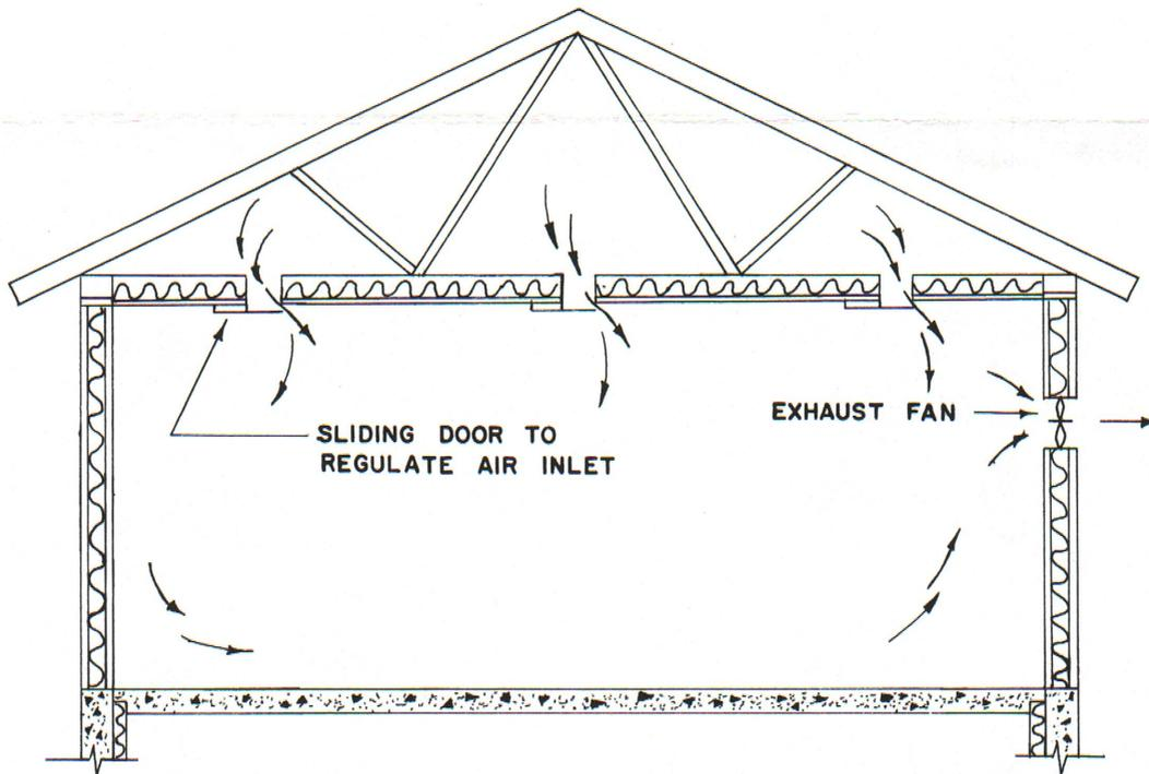
Fig. 4 FRESH AIR INLETS LOCATED IN THE CEILING
