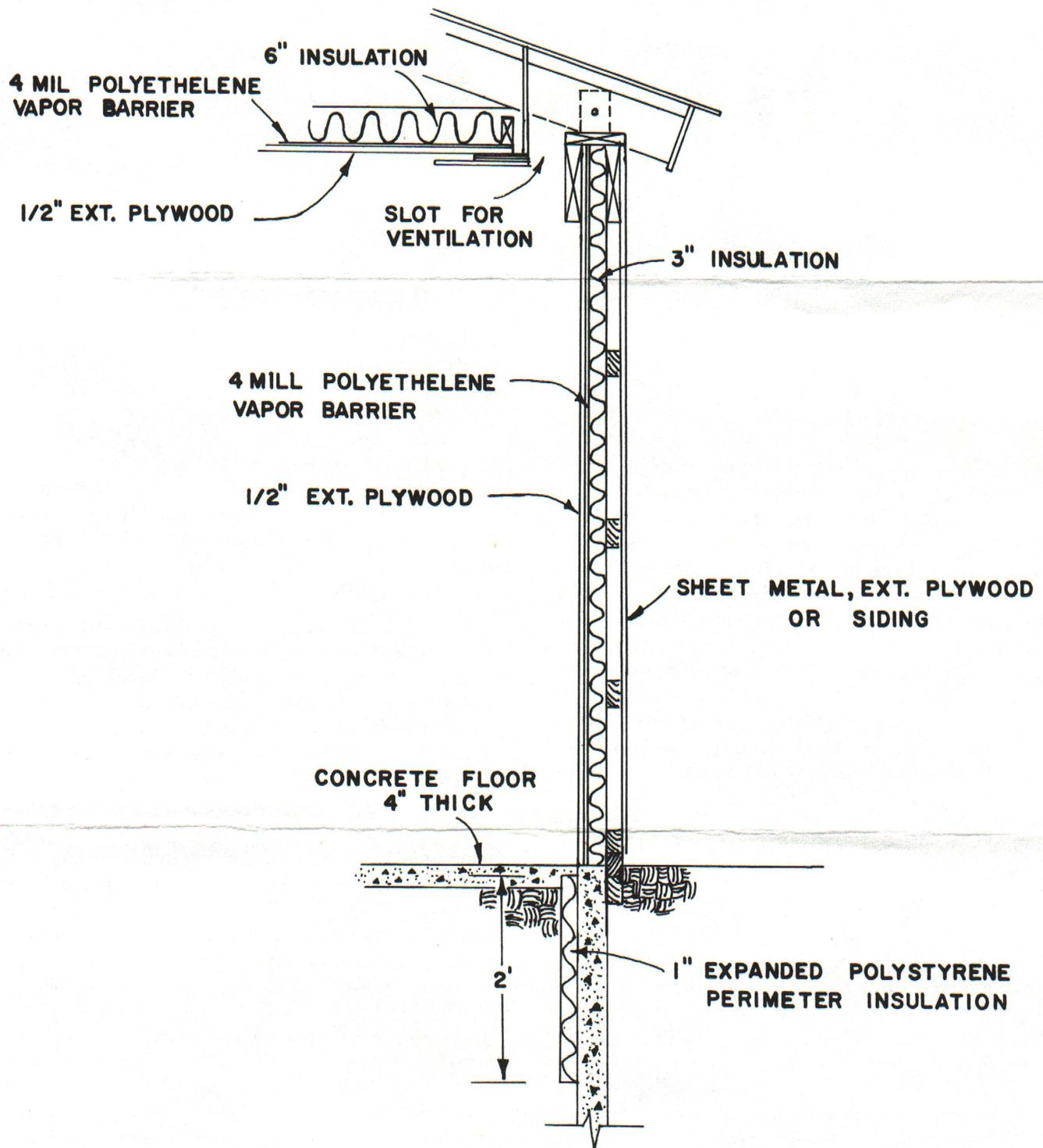
Fig. 1 CROSS SECTION OF FRAME WALL CONSTRUCTION
