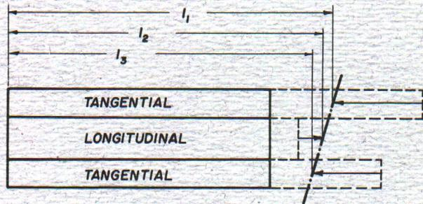
Figure 6. Warping of expanding three-ply panel due to unequal expansion of face and back veneers.
