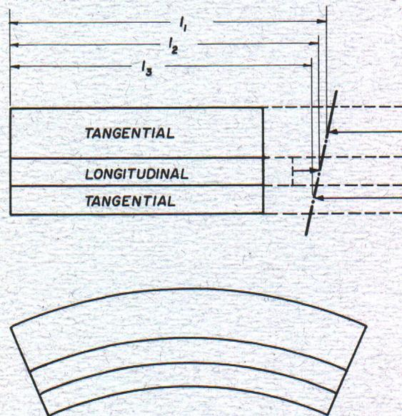
Figure 5. Warping of expanding three-ply panel due to unequal thickness of face and back veneers.
