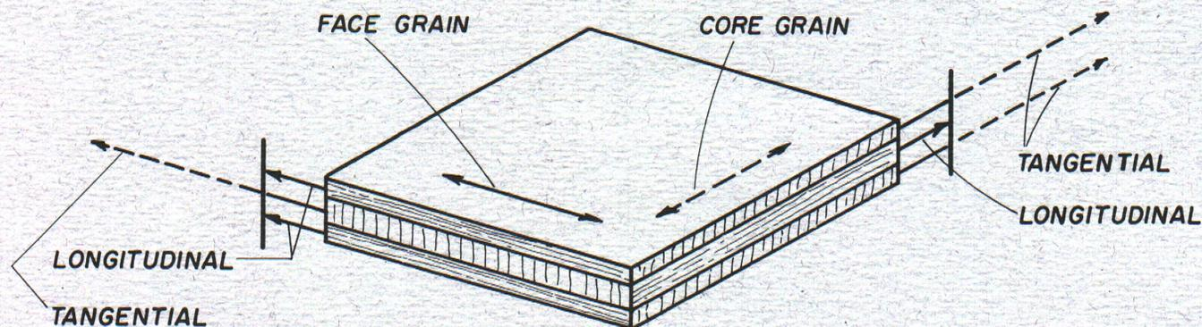
Figure 3. Mutual restraint of veneers in three-ply plywood.
