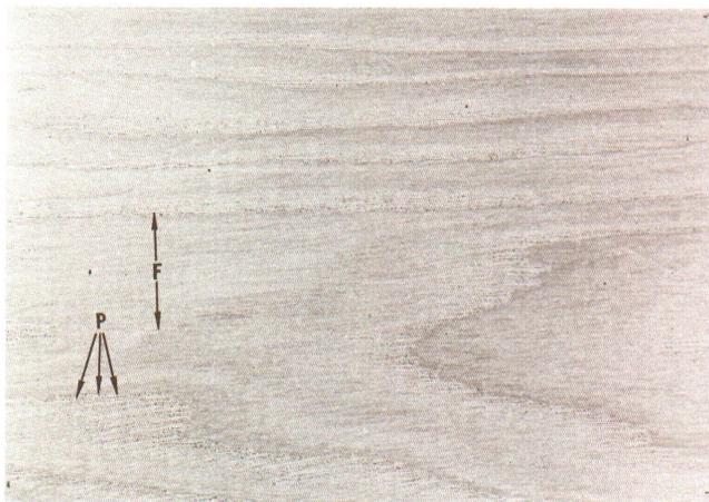
Figure 16—White Ash. Earlywood pores, P, poreless smooth areas, F.
