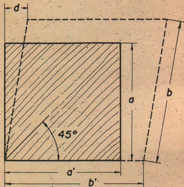
Figure 3. Swelling of square cross section when radial swelling is smaller than tangential swelling and annual rings oriented diagonally. ( $a = a'$ ;  $b = b'$ ). Values of "d" for square cross section with  $a = \frac{3}{4}$  inch: Silver Maple, 0.012 in.; Yellow Poplar, 0.009 in.; Yellow Birch, 0.006 in.
