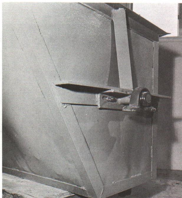
Fig. 1. Two methods of mounting bearings are illustrated in these pictures. Both are equally satisfactory. A 3 1/2" diameter hard rubber bottle stopper makes an ideal bumper. Rubber acts as a shock absorber and eliminates the noise caused by the tank dumping.
