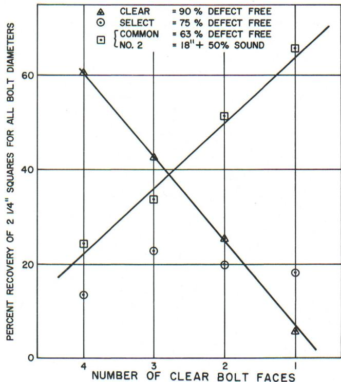
Overgrown knots, seams, and heavy bark distortions had a serious degrading influence on bolts up to 14 in. Bolts 14 in. and larger were able to grow enough wood over the defects so it was possible to produce some clear and select squares before defects appeared on the bolt's exposed surface.
