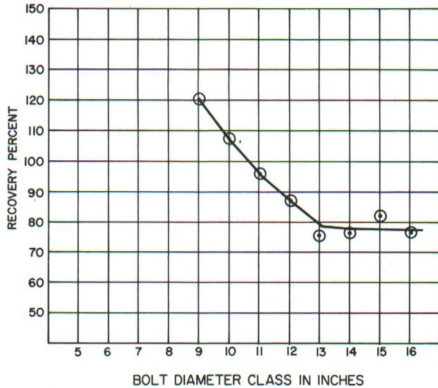
For bolt diameters from 13 through 16 in., recovery leveled off at approximately 78%. The average percent recovery for logs in this study was 86%. The waste occurred in the outside slabs, sawdust, and on a wedge-shaped center containing the pith.
