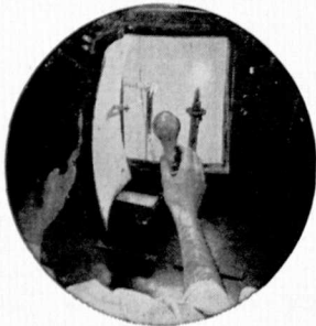
LIGHTING: Testing bulb light transmittance photometrically
