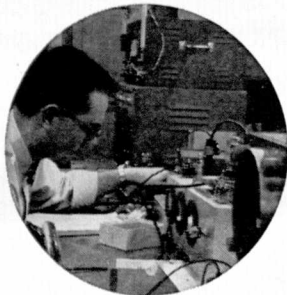
ELECTRONICS: Testing the characteristic of a counter tube
