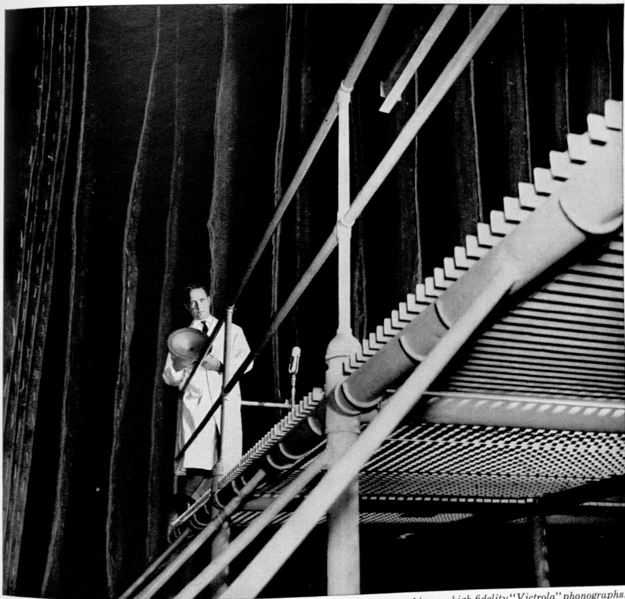
At David Sarnoff Research Center, Princeton, N. J., RCA tests one of loudspeakers used in new high fidelity "Victrola" phonographs.
