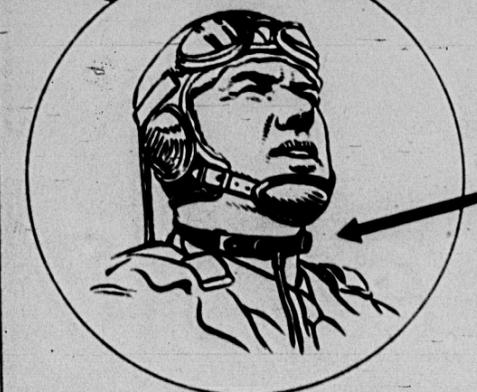
PILOT'S THROAT MICROPHONE (Radio-telephone transmitter)
