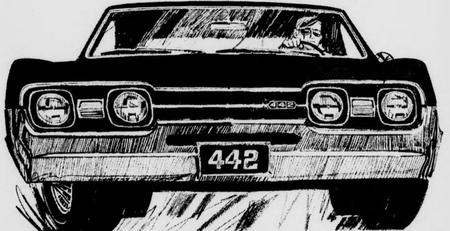
400 CID V-8. Full 115-inch wheelbase. Heavy-duty springs, shock absorbers, shaft. Sway bars, front and rear. High-performance axle. Dual exhausts. Beefed-up wheels. White-Line or wide-oval Red-Line tires. Bucket seats. Louvered hood. Higher oil pressure. They're all
