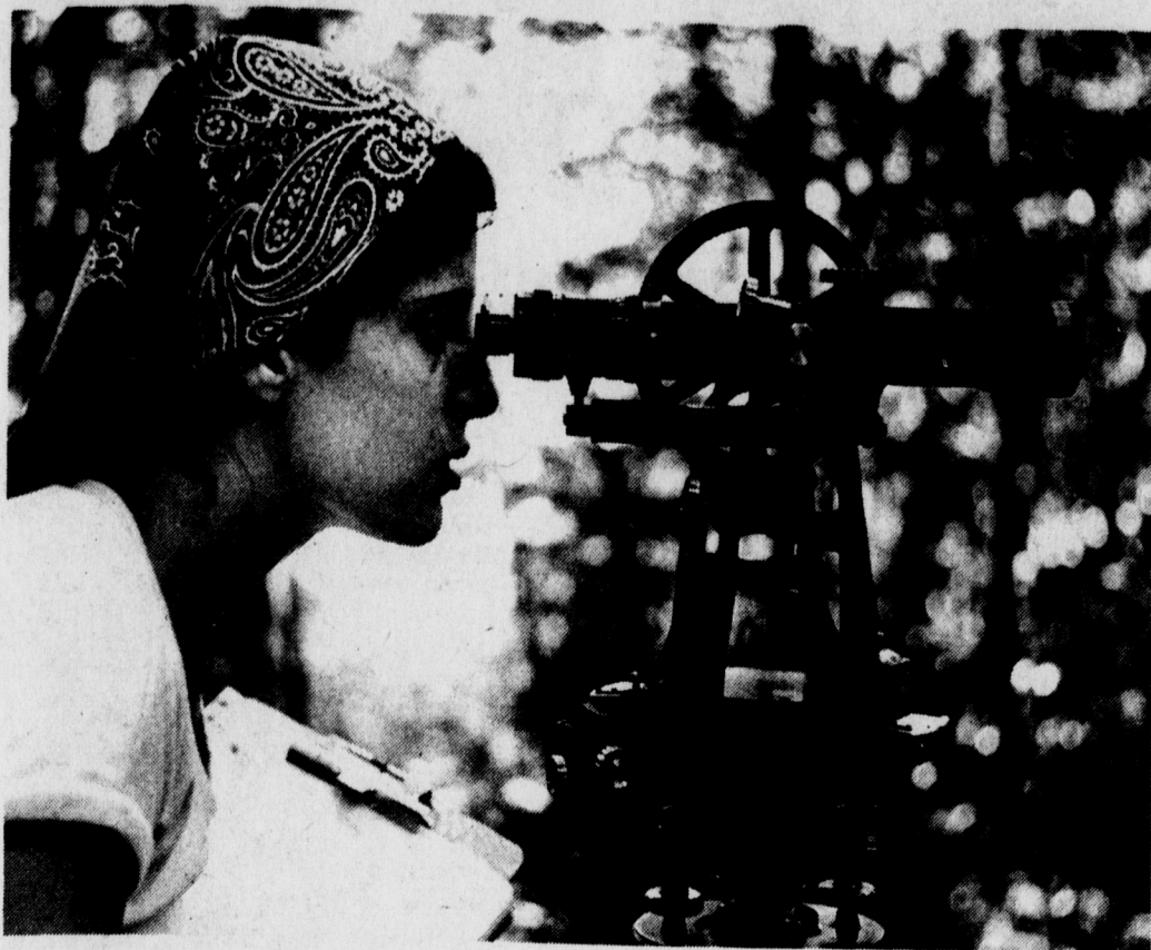
Sylvia Tiscornia operates the transit at the digging site as Richard Vorek holds the stadia rod. They are measuring the evaluation of the site.
