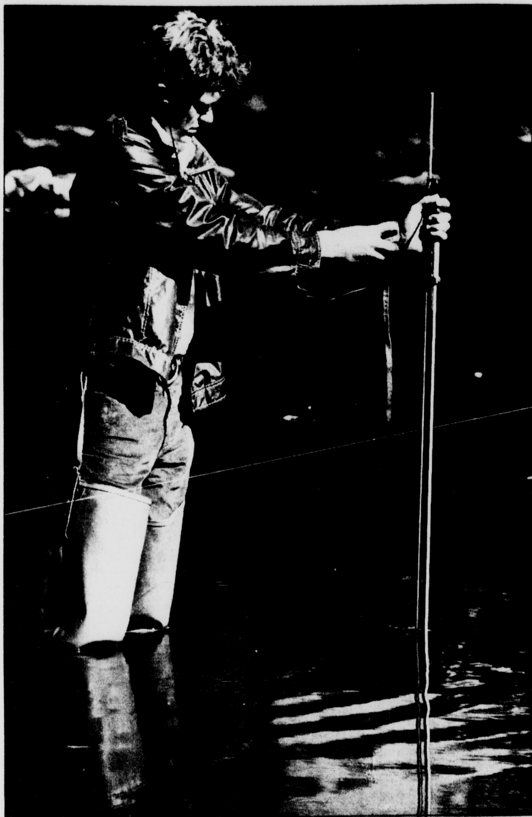
Steve Rheanme, a federal employee working for the U.S. Geological Survey team, is checking the water flow discharge of the Red Cedar River.
