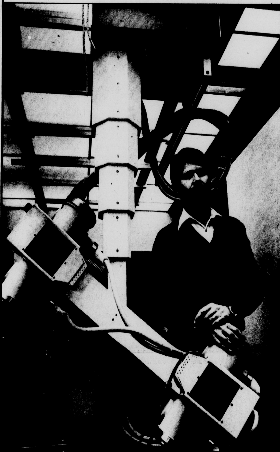
Herbert Reynolds, director of Systems Anthropometry research, stands near the stereo x-ray machine capable of measuring position changes of the human body with submillimeter accuracy using three-dimensional geometry principles.
